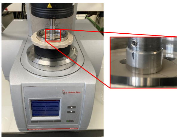
Figure 1: Rheometer with pin-on-disc test setup in Ringer's solution at 37 °C.
